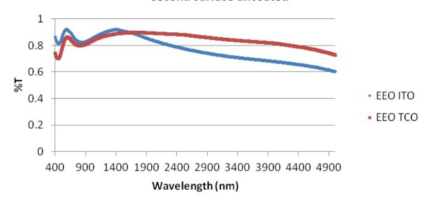
Transmission performance of the window will be improved and can be optimized for specific wavebands by AR coating the second surface
