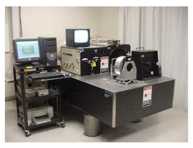
Figure 4. The overall system. The 1 inch output is dead center. The subsystem (rear view) is between the two Danger Laser placards. The 12 inch aperture collimator output and return mirror are on the right, unused in this application.
