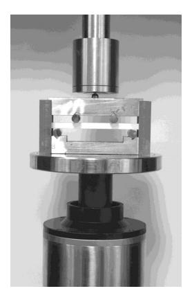
Figure 3: Four-Point Flexure Fixture loaded in the Instron Universal Tester (Photograph courtesy of UDRI Advanced Ceramics Group)
