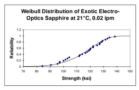
Figure 4: Plot of Probability of Failure vs. Strength.
