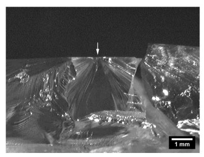
Figure 4: Typical Sample Fracture Initiation Site (Photograph courtesy of UDRI Advanced Ceramics Group)
