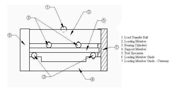
Figure 2: Diagram of "Size C" Four-Point Flexure Fixture
