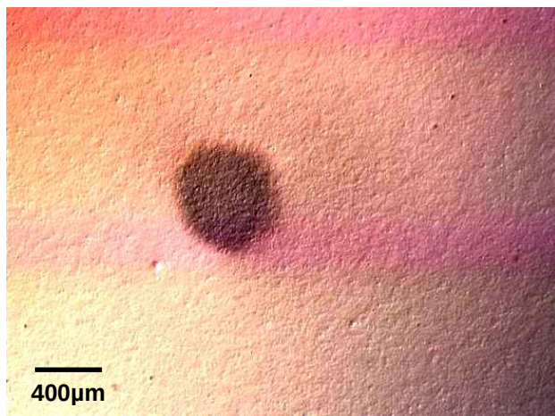
Figure 5. 0.02" diameter inclusion on the surface of inspection polished spinel sample. 50X.
