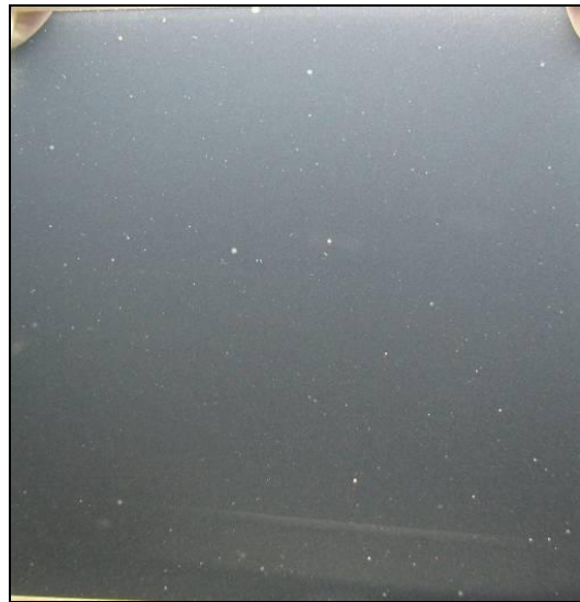
Figure 2. Representative photograph of inspection polished spinel material.
