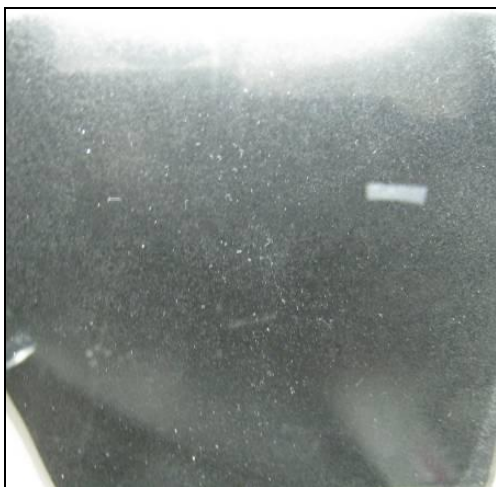
Figure 11. Photograph of polished spinel.
