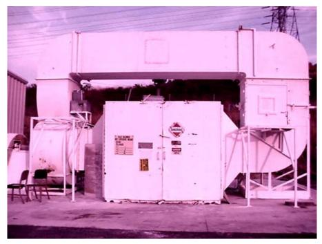
Figure 3: Example of a blowing sand test chamber (Photograph courtesy of National Technical Systems – Santa Clarita Facility)
