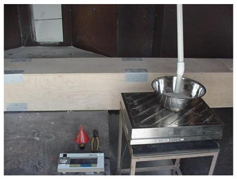
Figure 6: Example of a mass flow rate calibration set-up (Photograph courtesy of National Technical Systems – Santa Clarita Facility)
