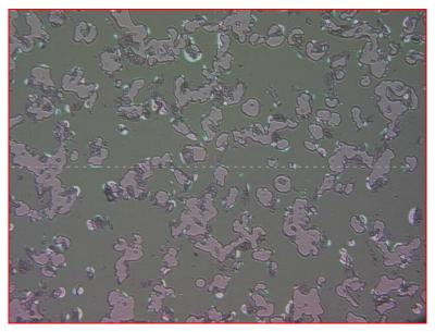
Figure 2: Typical Post-Test Visual Inspection Picture (Sample @ 200x magnification after 40 mph blowing sand)
