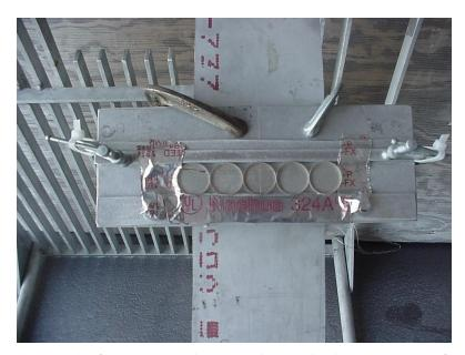
Figure 5: Example of a way to mount the test samples (samples shown are property of EEO) (Photograph courtesy of National Technical Systems – Santa Clarita Facility)
