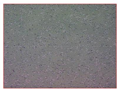
Figure 1: Typical Post-Test Visual Inspection Picture (Sample @ 50x magnification after 40 mph blowing sand)
